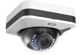
The IP Dome provides video streams in 4 MPx resolution with up to 30 fps. The impact, dust- and water-resistant IP67 / IK 10 housing protects against sabotage and vandalism. Due to the integrated IR LEDs the camera can be used at day and night. Access to the camera is possible any time via app.
