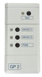
Active glasbreak detectors react more sensitively to glass breakage than passive ones. It is necessary to generate special test signals for each sensor type. Therefore, the glassbreak test instrument is equipped with different functions for active and passive glass breakage detectors. Via a piezoelectric disc on the front of the tester, the test signal is transmitted electromechanically into the pane and sensed by the glassbreak detector.
