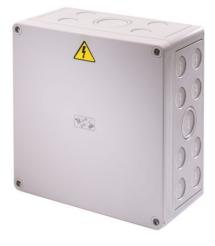
With the outdoor power supply, you provide the necessary voltage to all cameras and CCTV components that are installed outdoors. The output current (nominal current) is 4 A. Pre-cut perforations on the side of the housing enable customized openings for tidy wiring. The 4 outputs are individually fused and protected from overload and short-circuit.
