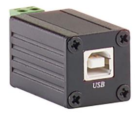
Use the interface converter to control a PTZ Dome Camera (TV7600 - TV7604) from your PC. The interface converter is connected to a USB 2.0 port at the PC and the dome camera is connected to the interface converter using a 2-core RS485 bus cable. You can operate up to 31 dome cameras with your PC. You connect one dome camera directly to the converter and connect the other 30 cameras to each other. The maximum transmission range from the interface converter to the last dome camera is 1200 meters.
