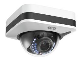
The IP Dome provides video streams in 4 MPx resolution with up to 30 fps. The impact, dust- and water-resistant IP67 / IK 10 housing protects against sabotage and vandalism. Due to the integrated IR LEDs the camera can be used at day and night. Access to the camera is possible any time via app.
